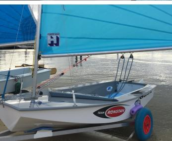
Based on the Griffin hull and 2015 National Champion Kalari 1188. Built with the latest technology to ensure its on weight but extra tough. Solid vacuumed bagged fibreglass.
