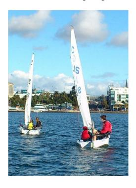
Keep boat flat Note the twist difference in jib and mainsail
